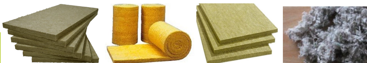
Figure 22 - Various forms of envelope insulation materials: batts, blankets, boards, and bulk
