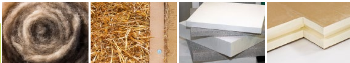
Figure 19 - Materials for building envelope insulation: sheep wool, straw bale, polystyrene and polyurethane
