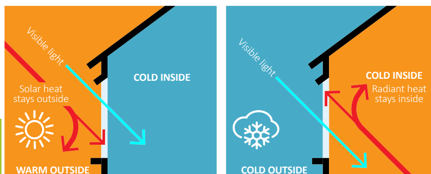
Figure 38 - Basic principle of how low-e layer improves insulation
